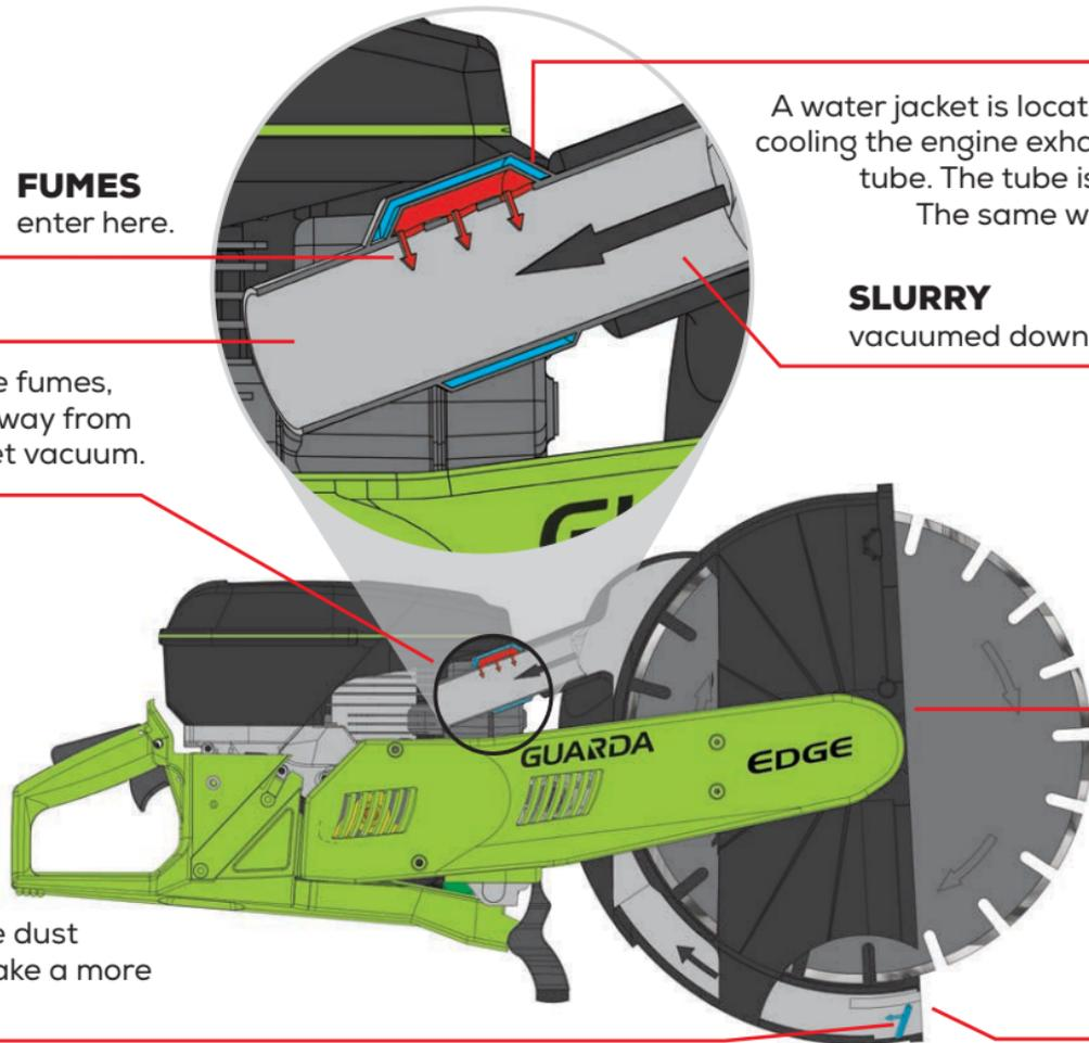
A water jacket is located around the exhaust ports for cooling the engine exhaust before it enters the vacuum tube. The tube is cool to touch during operation. The same water is used on the blade guard.
