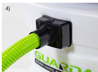
5) Connect 38mm/1.5" slurry hose to Edge Powercutter.
