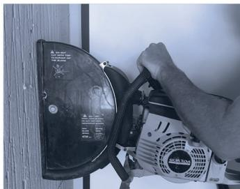
3. **During cutting.** Keep the blade guard against the cutting surface. To help achieve this the blade guard is designed to rotate within the vacuum shroud so that the orientation of the saw can change easily while keeping the guard against the wall.
