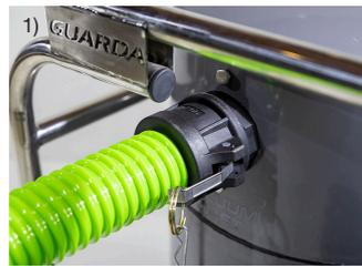
2) Connect 50mm/2" exhaust hose from Vacuum Generator to Slurry Interceptor using 50mm/2" camlock.
