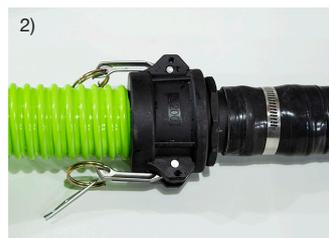
3) Connect 38mm/1.5" slurry hose to the Guarda Electric Exhaust Vacuum inlet. (hose length not to exceed 5m/15 ft between Guarda Electric Exhaust Vacuum & Edge Powercutter.
