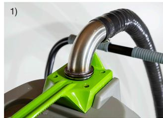
2) Connect the 50mm/2" exhaust hose to the Kevlar connecting hose to exhaust the Edge engine fumes outside in a well ventilated place. You can extend the 50mm/2" Guarda Exhaust hose to a maximum of 60m/200feet.
