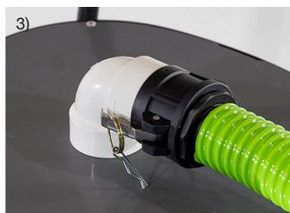
4) Connect 38mm/1.5" slurry hose to Slurry Interceptor vacuum inlet. (Hose length not to exceed 5m/15 ft between Slurry Interceptor & Edge Powercutter).
